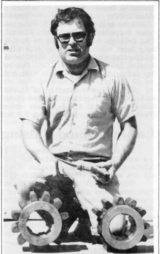
Master Machinist Edward L. Horne poses with the old and new rotation gear that he built from scratch so our prized crane can be returned to duty.
